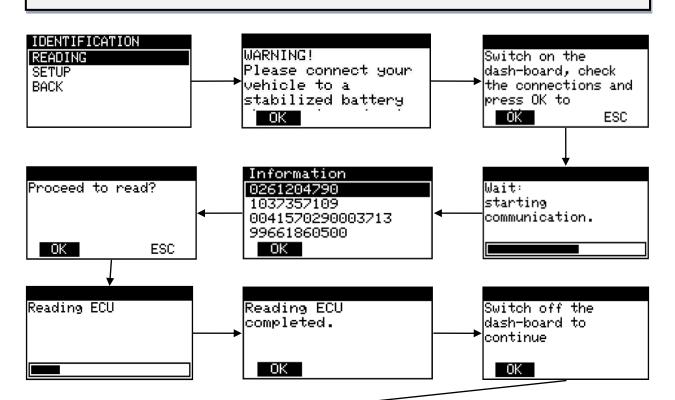
MyGenius tool has now properly read the ECU. Unplug the OBDII cable from the car and connect the USB cable to the MyGenius device and to the PC. To export the READING file from the device follow the instructions of the chapter *FILE DOWNLOAD* on page 13.
