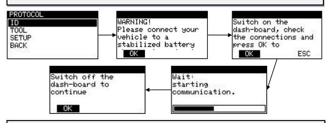
MyGenius tool has now properly identified the ECU. Unplug the OBDII cable from the car and connect the USB cable to the MyGenius device and to the PC. To export the ID file from the device follow the instructions of chapter *FILE DOWNLOAD* on page 13.
