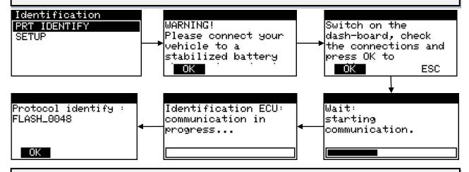
MyGenius has properly identified the correct serial protocol for your car. Click OK and select WORK, depending on the protocol the device will be able to perform the reading or the identification only of the ECU software.
